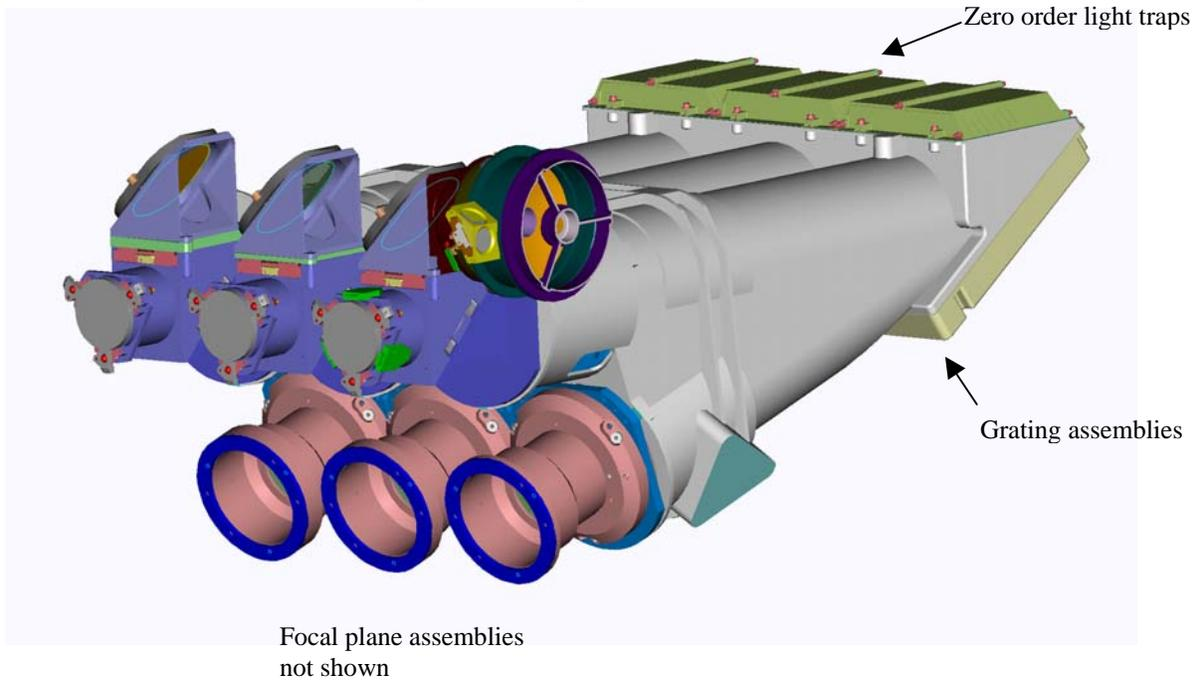
Figure 5: F/1.8 telescope and collimator section view
