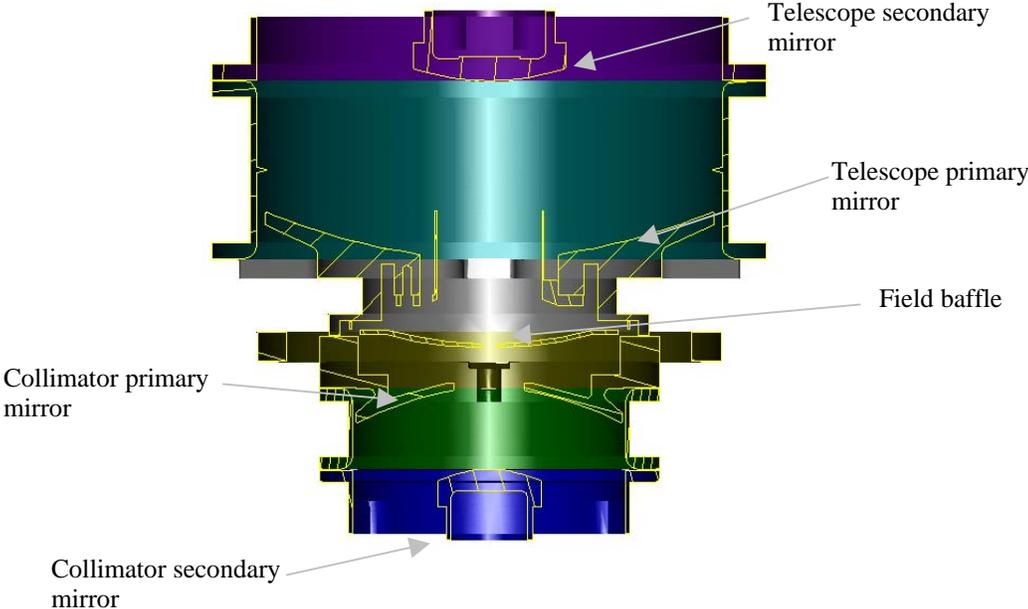
Figure 6: Entrance baffle/calibration sub assembly (science mode shown)
