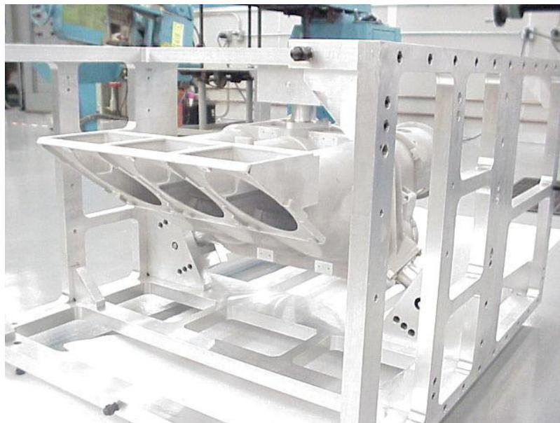
Fig. 4. The flight spare optical bench housing mounted in the bench assembly/alignment fixture during a check fit at the Hamilton Sundstrand facility in Long Beach, CA.
