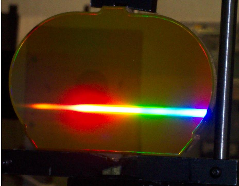
Fig. 9. A flight diffraction grating mounted for Bi-Direction Reflectance Distribution (BRDF) measurements to independently verify the parts scattered light properties.
