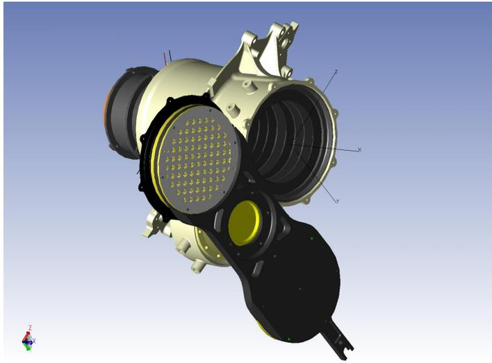
Fig 6. The OCO instrument baffle calibration assembly stray light analysis model. The calibration paddle is shown in the normal science mode with the aperture open. Rotation of the paddle 90 degrees clockwise places the instrument in the solar calibration mode.
