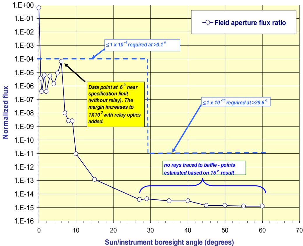
Fig. 7. Simulated stray/scattered light reaching the a-band spectrometer entrance slit as a function of instrument/sun angles. The specification is that less than  $1 \times 10^{-4}$  of the scene radiance 0.1 degree outside the instrument field of view reaches the detector. At angles greater than 29.6 degrees the requirement becomes less than  $1 \times 10^{-11}$ .
