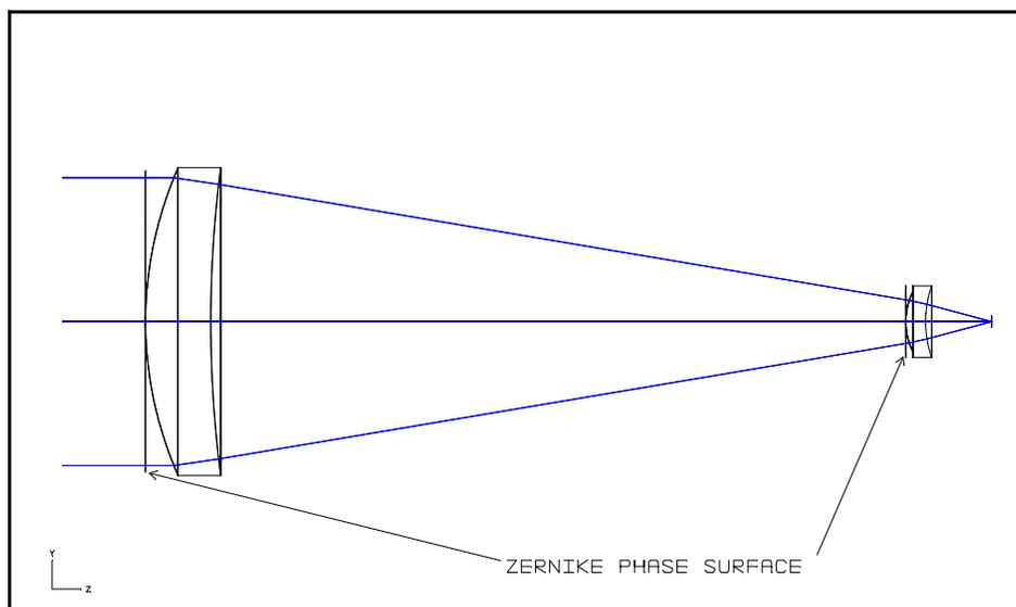
Fig. 8. Zernike phase surfaces were inserted into the nominal prescription allowing as-built performance assessment.
