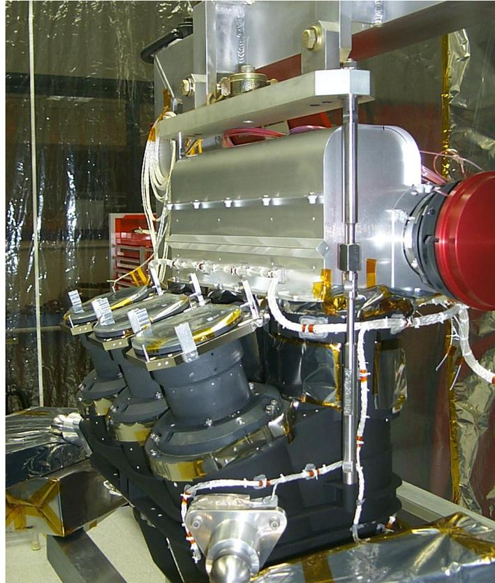
Fig. 3. Showing assembled optical bench in the area of the telescope. A tooling cover (red) is covering the telescope aperture at the right center of the picture. A temporary relay shroud (bright aluminum piece behind the telescope) will be replaced with flight hardware after the focal planes are aligned and focused. The flight detector assemblies attach to the three-camera lens exit flanges at the lower left. Image credit NASA/JPL.
