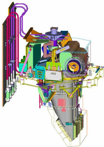
Fig. 1. The OCO Primary Instrument Assembly (PIA). The thermal shroud and instrument deck are transparent to view the internal optical bench. The heat rejection radiators and connecting heat pipes on the left of the view are the only PIA components external to the spacecraft. The telescope views the Earth through an opening in the side of the spacecraft.
