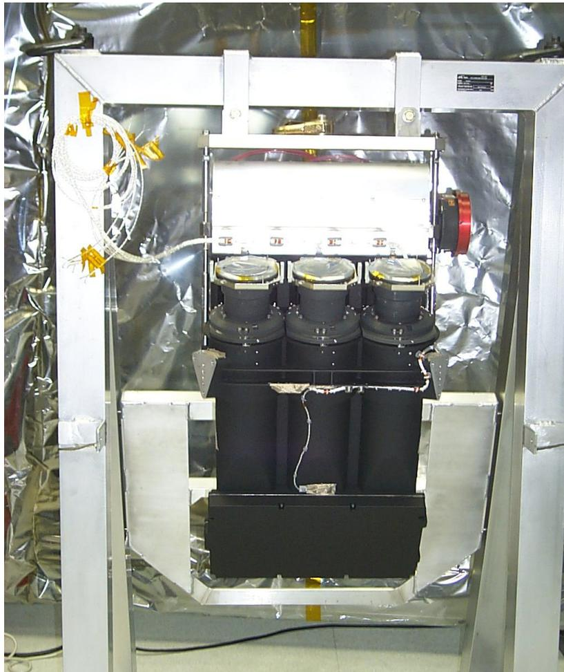
Fig. 5. Flight optical bench housing with collimator and camera lens assemblies aligned and pinned in place. The spectrometer diffraction gratings are under the black cover at the bottom of the bench. Image credit NASA/JPL.
