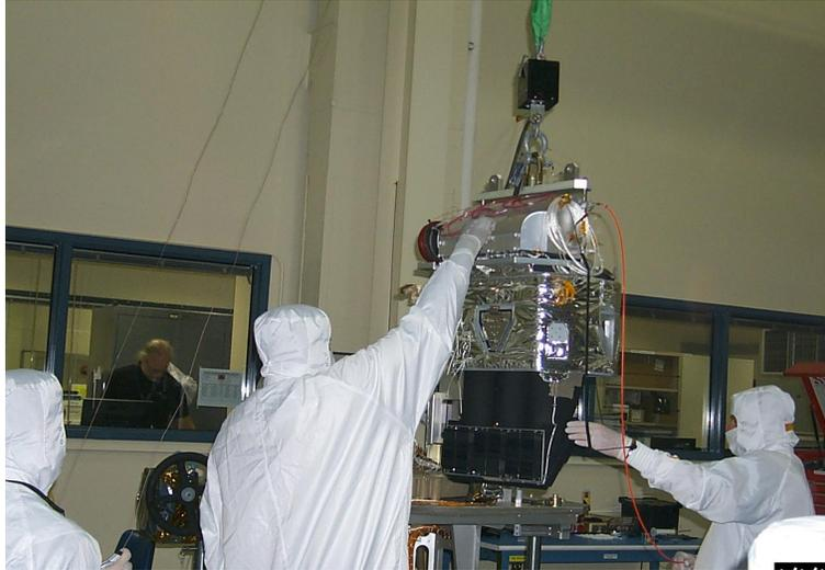
Fig. 2. The OCO Instrument Assembly in the JPL High Bay. The complete Optical Bench Assembly, with mid-thermal shroud section attached, is shown. The entrance telescope is pointing toward the control room window (left). Image credit NASA/JPL.
